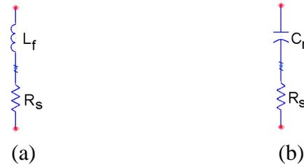
**Figure 3 (a) Forward and (b) reverse bias equivalent circuit of the PIN diode**
