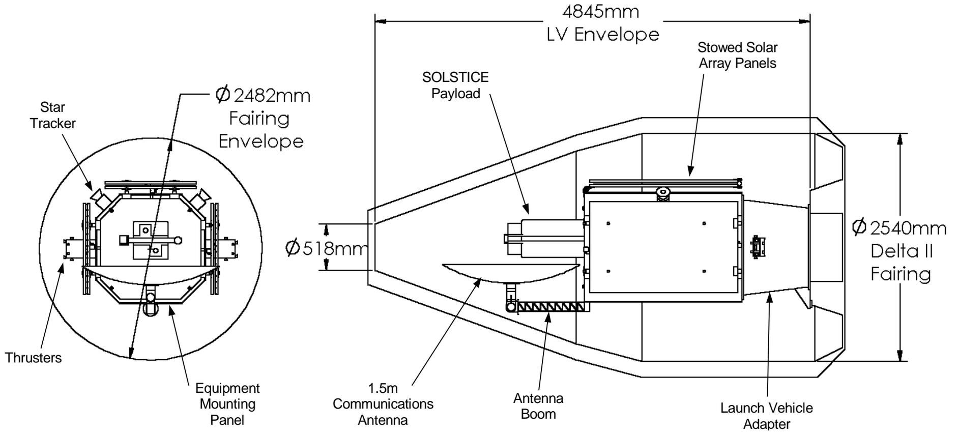
Figure 3.1: Stowed Configuration of Sunstroke
