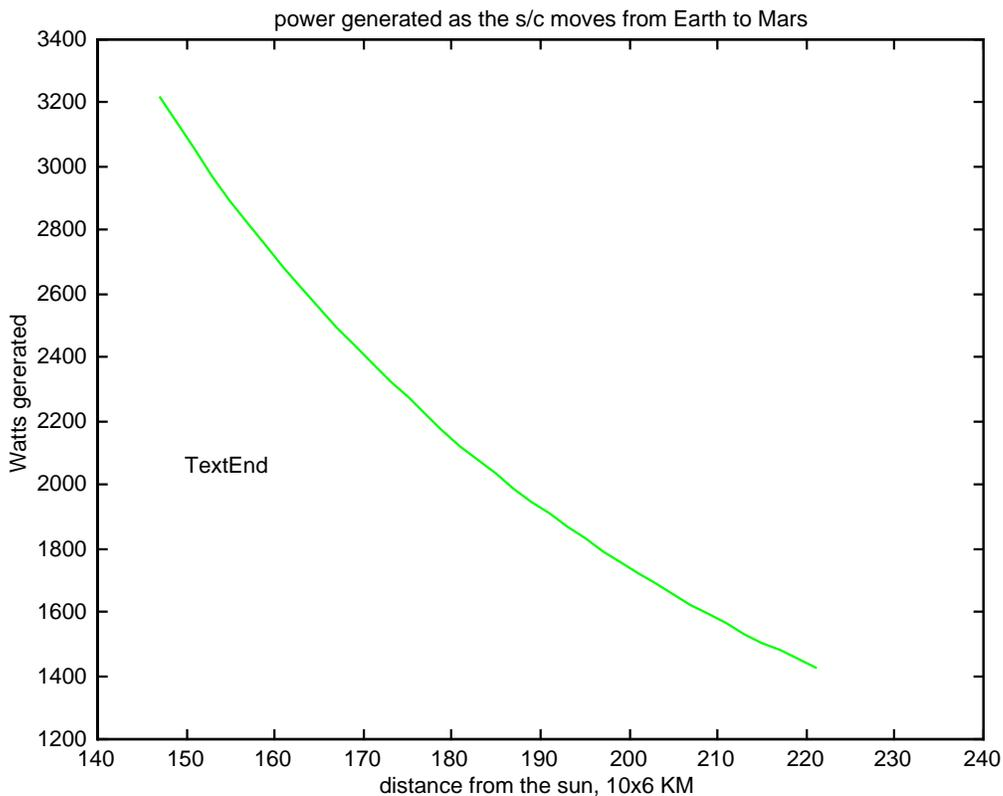
**Figure 6.4. Power as Spacecraft Moves from Earth**
