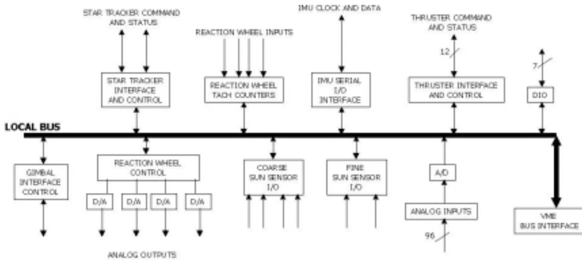
Figure 8.3 Attitude Control Interface Card Functional Diagram
