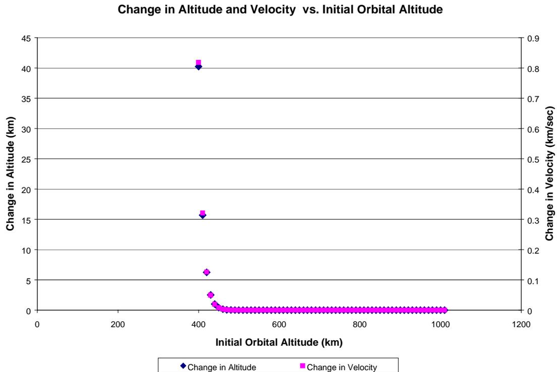
Figure 2.2: Effects of Aerodynamic Drag on Altitude and Velocity
