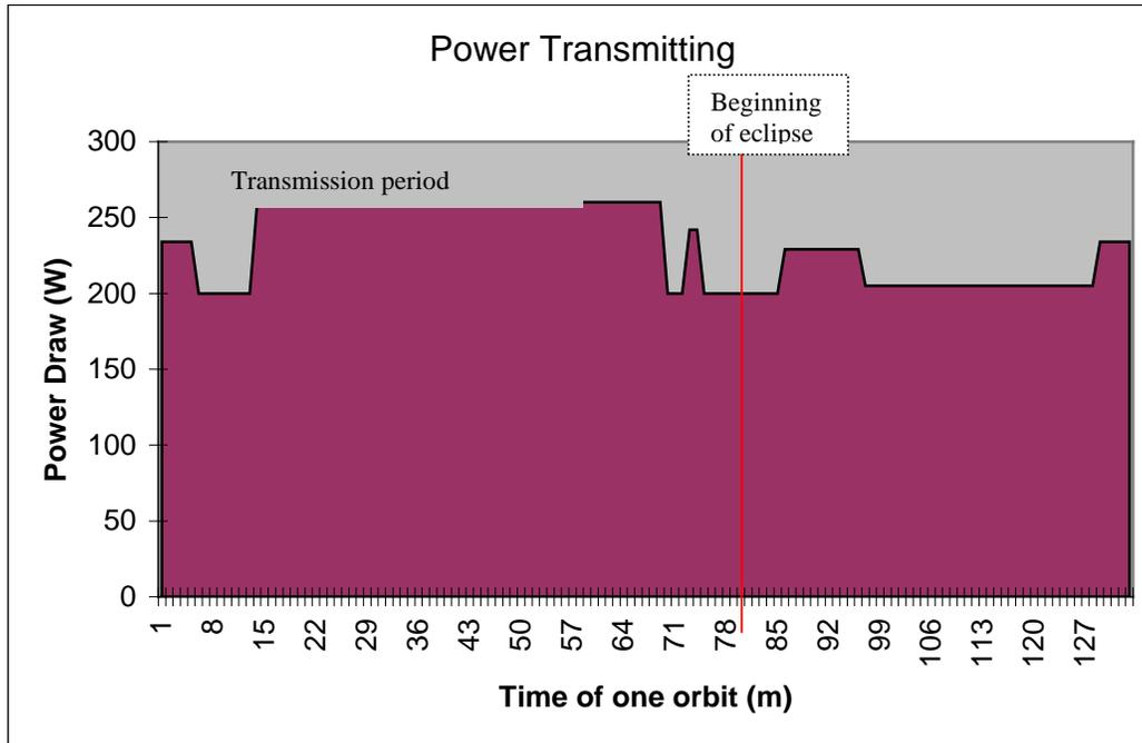
Figure 6.7. Power Profile while Transmitting
