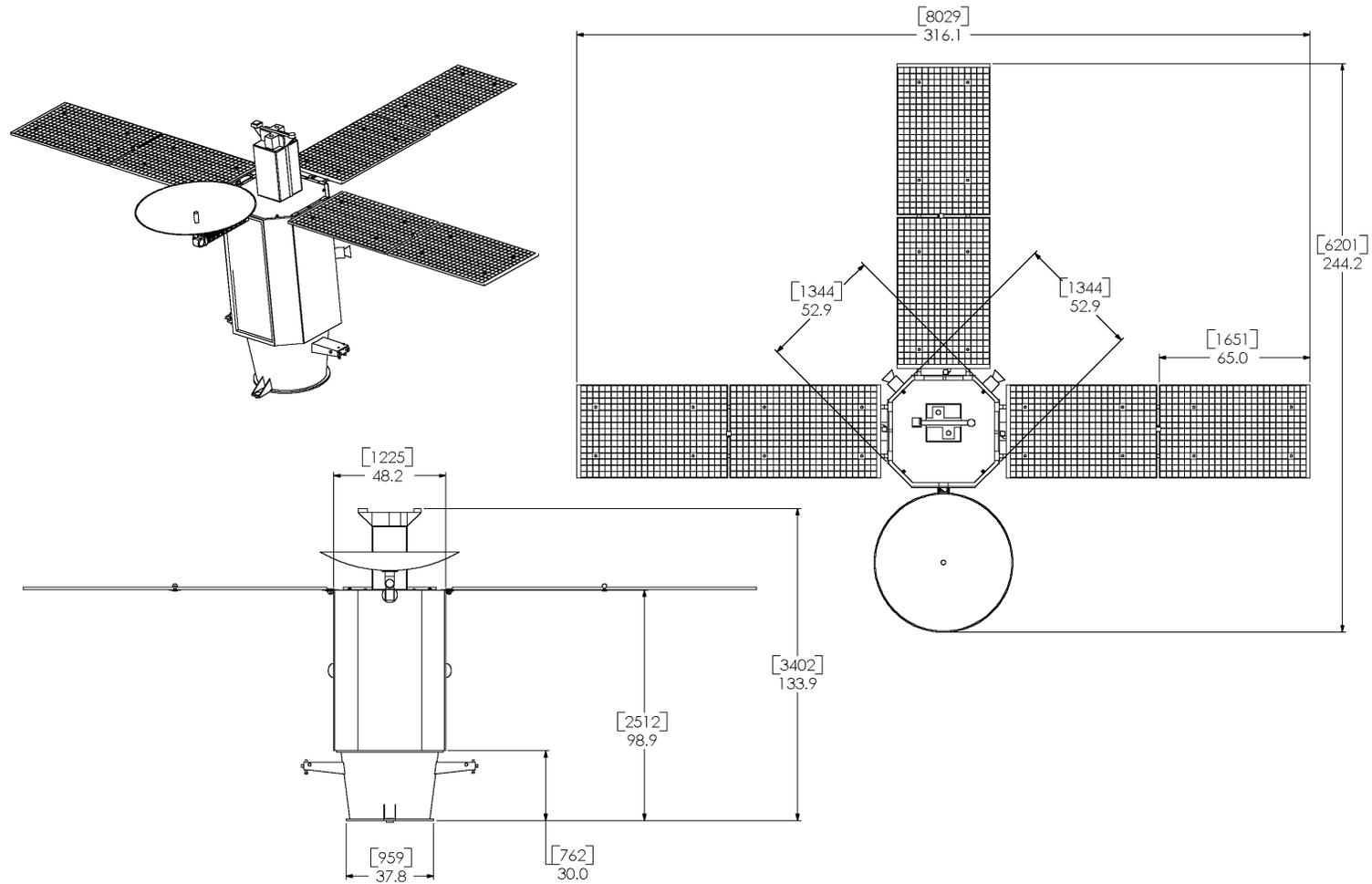
Fig 1.2 Sunstroke Envelope Drawing
