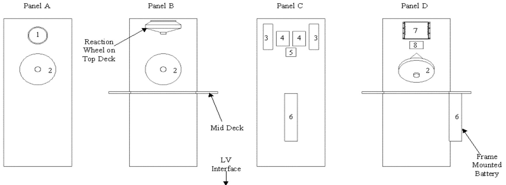
Figure 3.4: Layout of Sunstroke's Internal Packaging Arrangement
