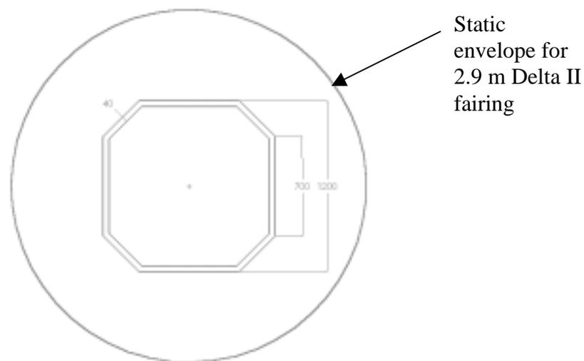
**Figure 3.5: Modified square cross-section used for Sunstroke.**
