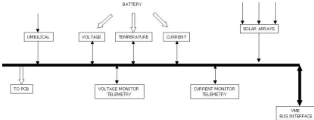
Figure 8.4 Charge Control Board Functional Diagram
