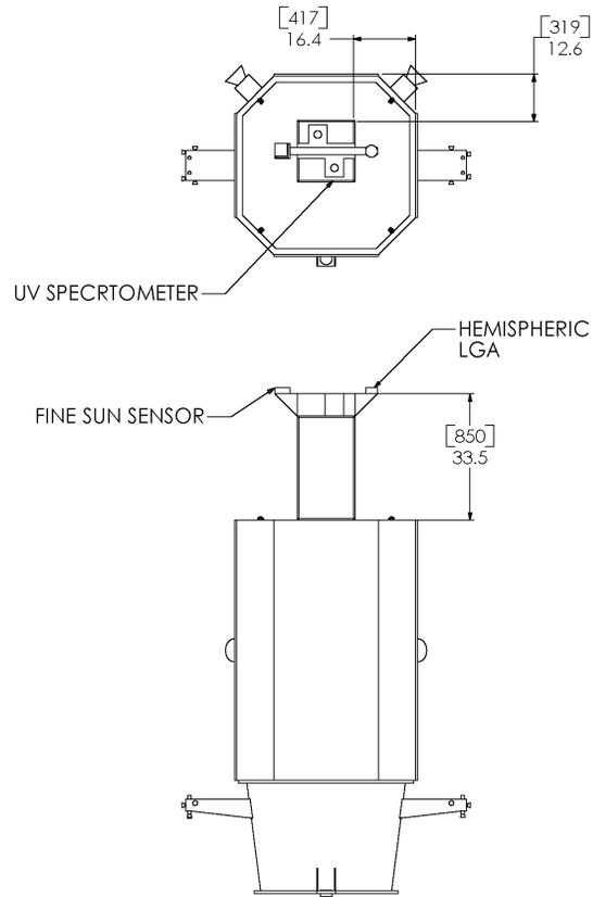
Fig 1.3 Instrument Mechanical Interface
