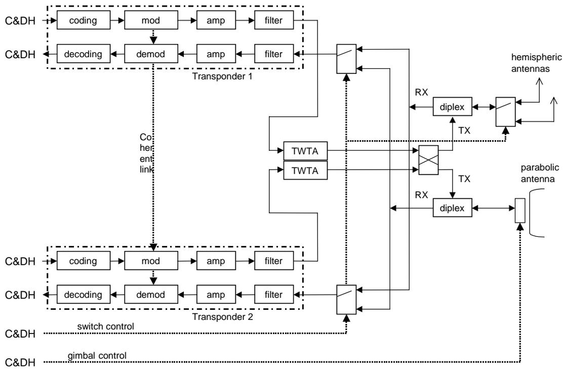
Figure 9.1 Telecomm Block Diagram
