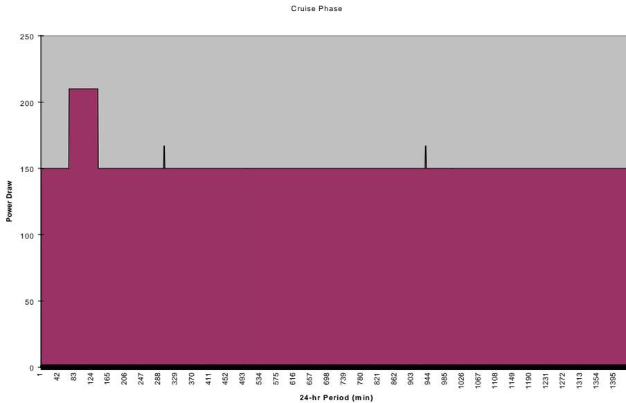
**Fig 1.5 Power Profile during Cruise**
