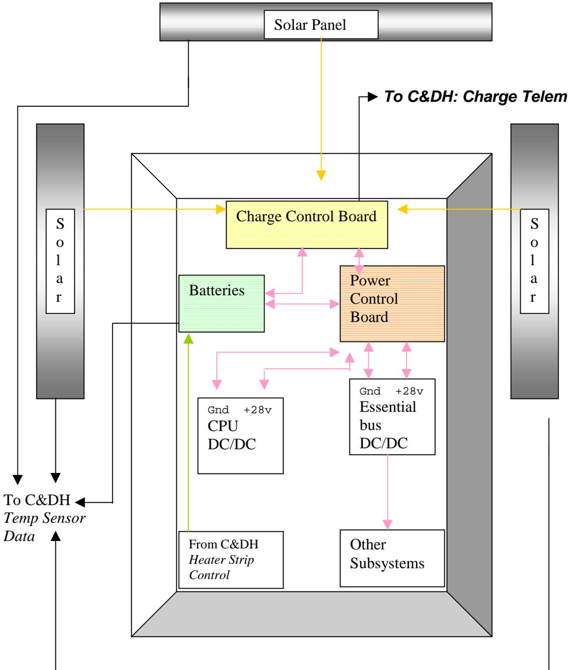
Figure 6.1. Power Block Diagram
