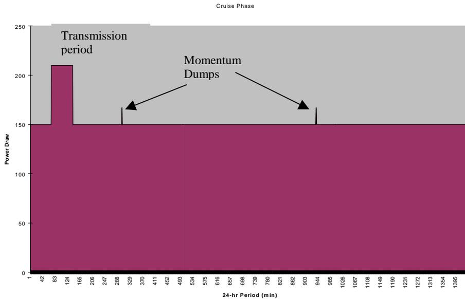
**Figure 6.5. Power Profile during Cruise**
