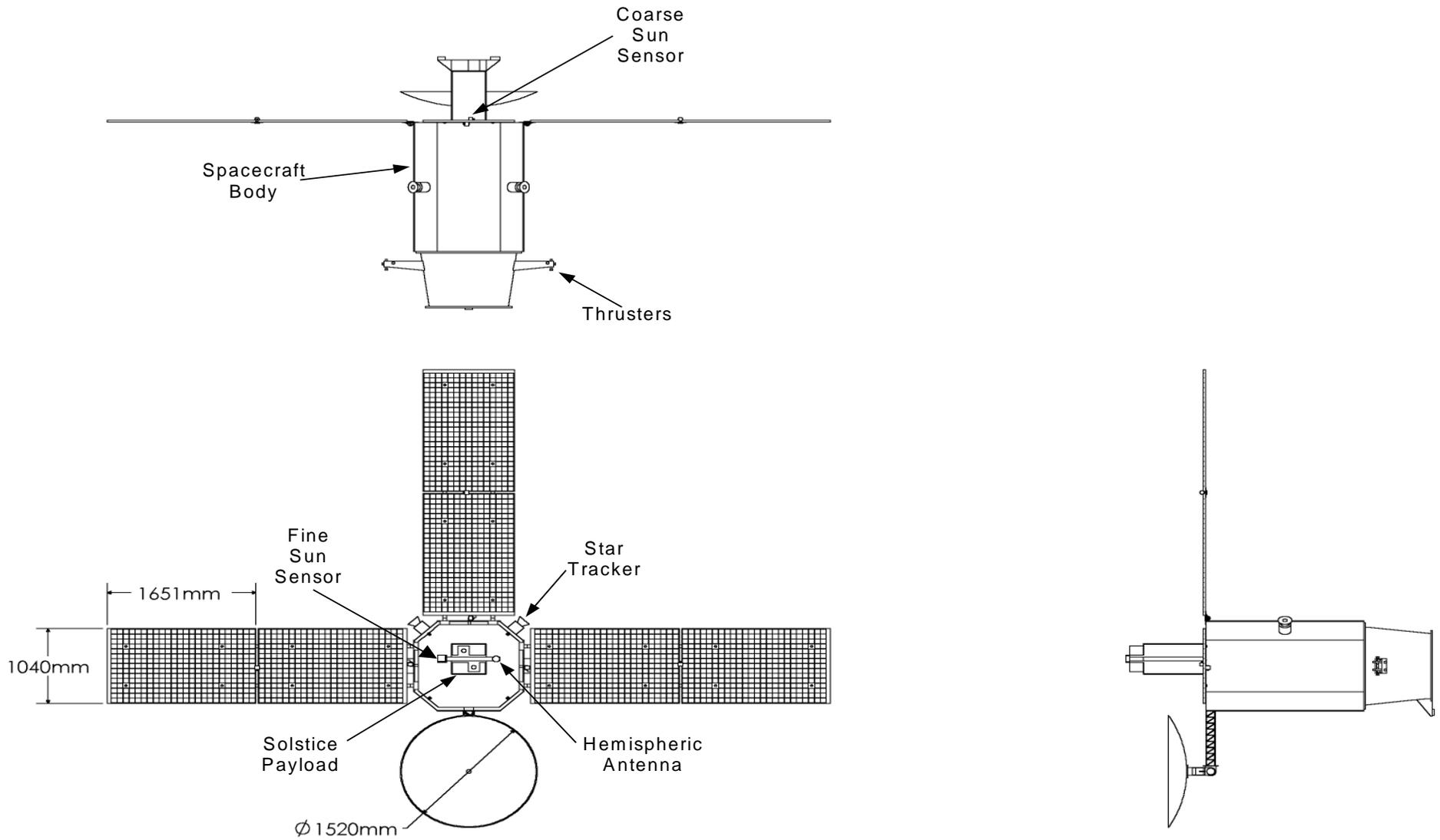
Figure 3.3: Deployed Configuration of Sunstroke
