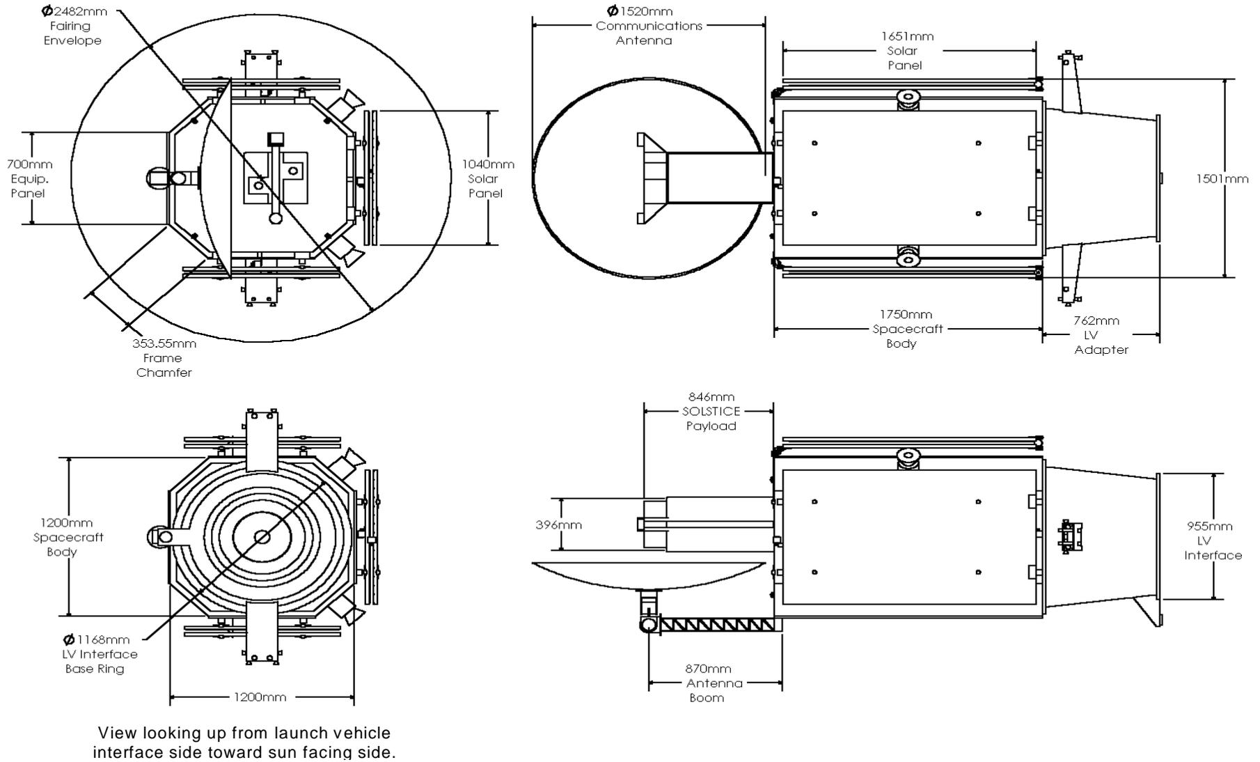
Figure 3.2: Stowed Configuration of Sunstroke – Additional Views
