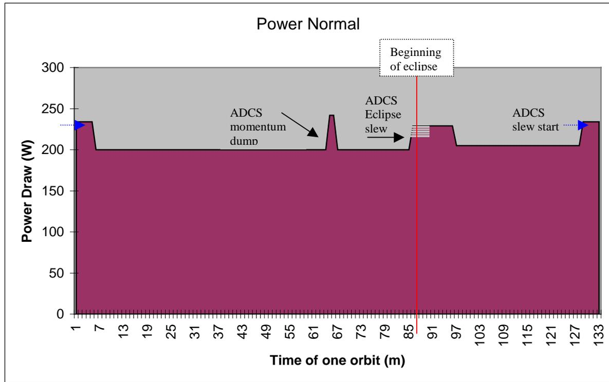
Figure 6.6. Power Profile during standard orbit
